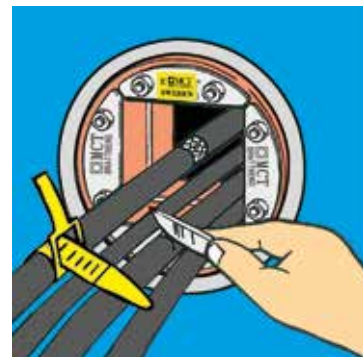
3 Pull the cables to final position. Mark cable 30 mm (1.18") from front edge of frame. Remove cable sheath 5 mm (0.2") on either side of the line.
