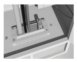
19. For reinstallation remove the PTG 40 wedge.
