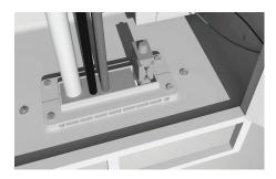
13. PTG 40 wedge can be inserted from both sides of the frame depending on access or client specification.
