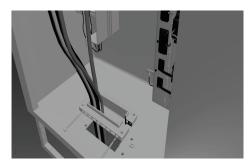
15. Install the preterminated cables between the two halves of RFCS frame.
