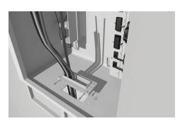
16. Screw together the two halves with middle gasket fixed on one half of the RFCS frame.
