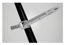
3. Use the cable selector to find the exact diameter of cable by wrapping around the circumference of cable.
