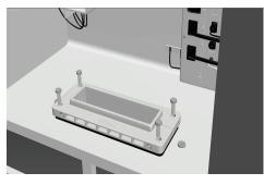
2. Install the frame and gasket directly on the cabinet cutout before installing the cables.
