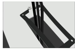
17. Install all preterminated cables aftermaking an angular cut in the gasket and secure the gasket on cabinet cut out.
