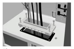
18. Fix the RFCS frame together with back gasket on the cabinet cutout by tightening with mounting hardware.
