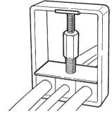
2. The packing tool keeps the cables and blocks into place.
