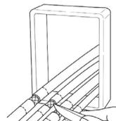
2. Remove the cable sheath between the two lines in the middle.
