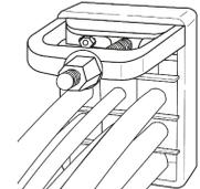
2. attach the endpacking puller to the bolts with the nuts.
