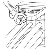
3. Tighten the bolt on the puller, the endpacking slides out.
