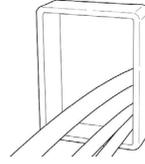
1. A cable separator tool keeps away the interference of cables.
