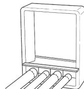
4. Complete the row of E-blocks and insert the stayplate. Repeat on the rest of the cables.
