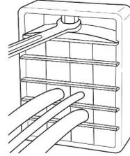
Tighten the bolt on the compression plate with the quick release spanner.
