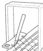
1. Pull the cables to final position. Put the EMC marking template in the frame with the yellow label facing you. Mark the cables.
