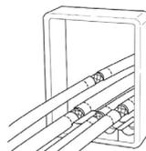
3. Push the exposed part of the cable screen so it is positioned over the metal sheet in the E-Insert blocks. Ensure all the insert blocks having the yellow "E" markings facing you.
