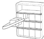
2. Ensure the tweezers blades protrude at least 35 mm outside the block. Insert the tweezers blades in the frame
