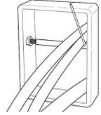
2. Position the cable separator within the frame and tighten it up with the metal bar enclosed.
