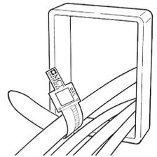
2. Put the measuring strip around the cable.
